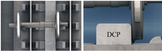
Fig. 1. Derailment Containment Provision (DCP)
