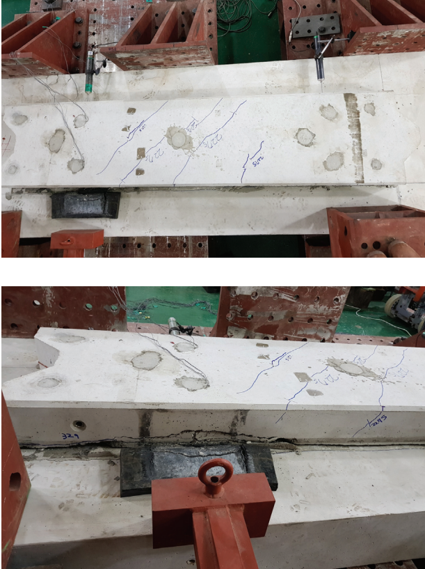
Fig. 11. Crack Shape of Specimen Loaded at Anchor Connection
