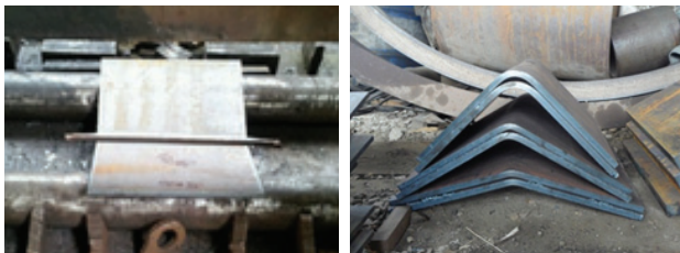
Fig. 2. Press Fabrication and Bending Degree
