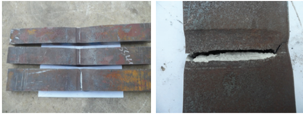
Fig. 9. Fracture of Mid-Jacking Calibration (S30-T-30 Specimen)
