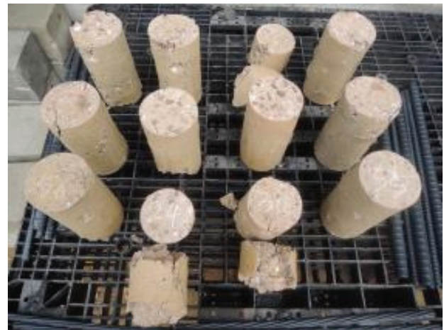
Fig. 1. Specimens Failure Under Water Cooling
