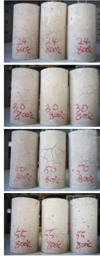
Fig. 6. Fire Damaged Specimens (Target temperature: 800 °C)
