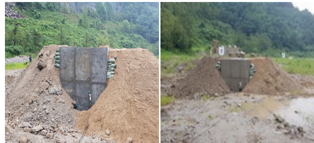
(a) Normal-strength concrete (b) High-strength concrete Fig. 8. Explosion Test Setup
