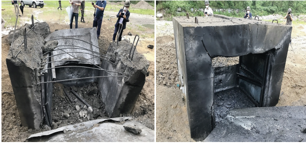
(a) Normal-strength concrete (b) High-strength concrete
