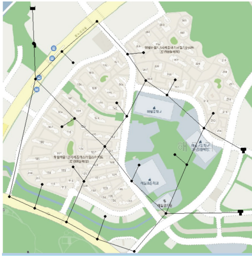
(a) Water distribution network (EPA-NET)
