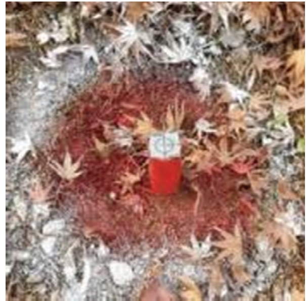
Fig. 3. Installed Pile For Check Point
